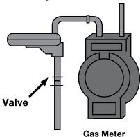
To turn gas off, give the valve a quarter turn in either direction. When the lever crosses the direction of the pipe (see below) the gas is off.
